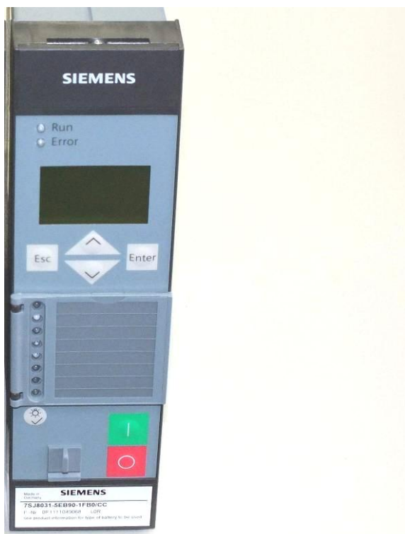
picture 3 Protection Relay 7SJ80 without visible corrosion phenomena or deposits after the corrosive test Ke
