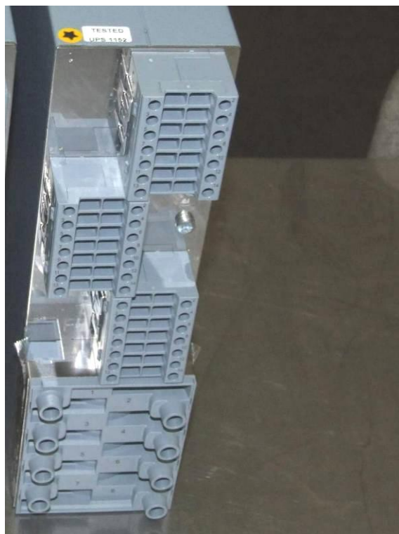
picture 2 Protection Relay 7SJ80 before the corrosive test Ke
