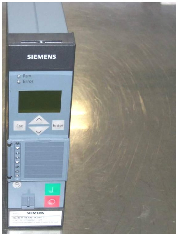
picture 1 Protection Relay 7SJ80 before the corrosive test Ke
